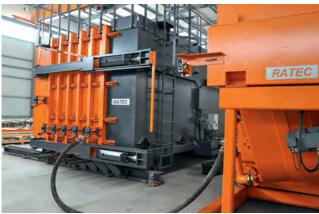
Hydraulic battery mould with pump car
