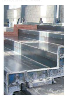
SPB for fixing staircase moulds
