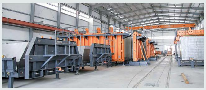
Module and roof shelling in the newly built plant in Ica
