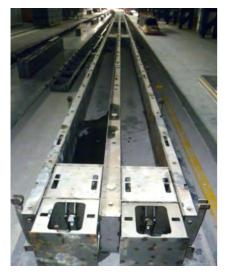
Pile shuttering based on the SAS-MF
