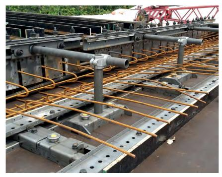
Easy Form in combination with UAR adapter for continuous reinforcement and upstand in the element
